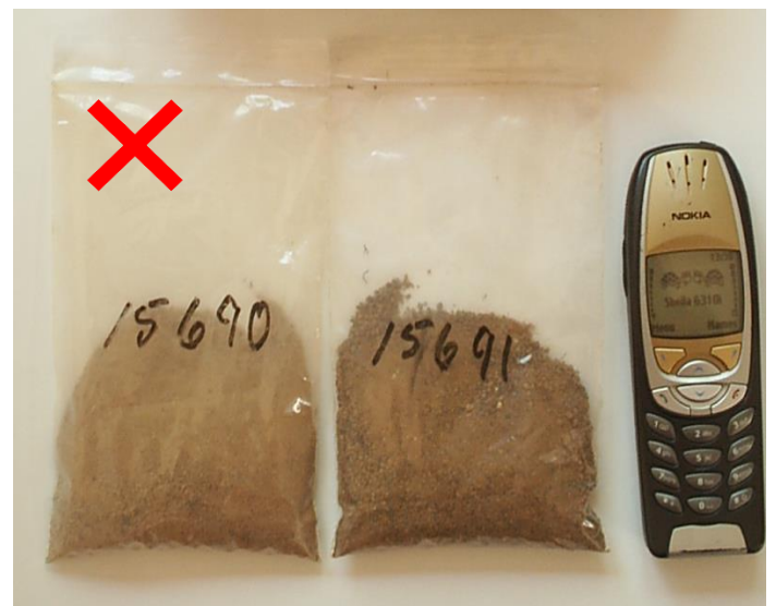
Wrong amount of soil
